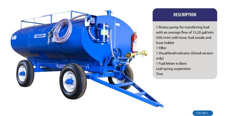
Agricultural tank trailer for transport of diesel or water, "U" beam chassis in carbon steel, independent of the tank and 5th wheel steering type. Semi elliptical tank equipped with wave breaks, manhole and drawer register. Pump drive system can be driven by combustion engine or tractor power take-off.
